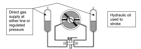
This method applies direct gas pressure onto the oil being stored in the reservoirs, therefore, forcing the oil through the actuator controls to stroke the actuator. This system will also incorporate a manual override in the form of a manual hand pump installed in the normal hydraulic circuit. Some systems have a 3rd reservoir, which is used only for the purpose of storing gas pressure in the event of a gas supply being lost.
