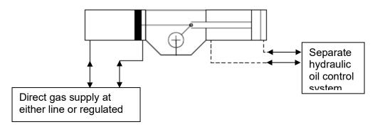
This method only applies direct gas pressure onto the pneumatic cylinder side of the actuator to stroke the actuator. This method of operation is used during normal modes of operation. However there is a separate hydraulic manual override control system that will, in the event of gas pressure being lost, provide an alternative method of stroking the actuator.
